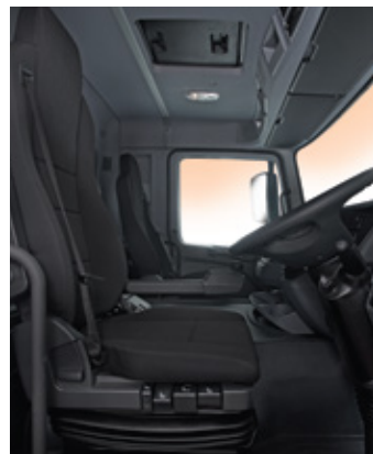
The optional air-sprung suspension seat with lumbar support and lateral contour adjustment offers supreme comfort for driving. Its ventilated seat made of sturdy velour and Alcantara is able to get rid of heat and moisture.
