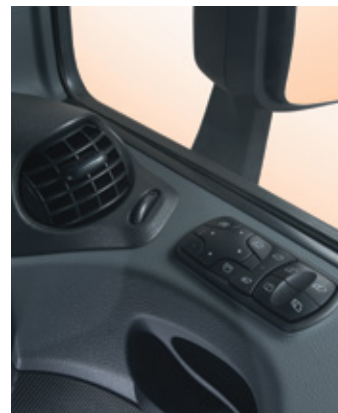
The ball-type air vent provides a flow of cool air for the driver in the tropical climate. The illuminated switches for the central locking system, power windows, mirror adjustment and mirror heating system can be easily found.
