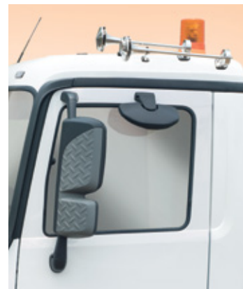
Better visibility with better safety. The wide angle mirror and new exterior mirror to enlarge the driver's field of view to the predecessor model. Also with the high top and rotating beacon lamp for better visibility even if the Actros was operated in the middle of the night.
