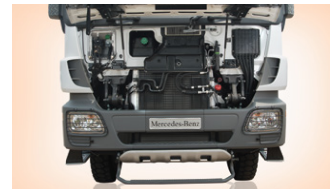
Ease of maintenance can be done by opening the front grille. This includes all maintenance for electric box, oil measurement, water cooling, wiper fluid and clutch oil.
