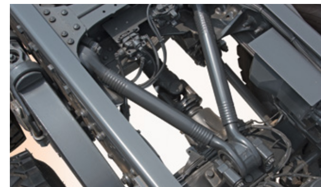
Innovative rear axle V-Control Arms are used in the Actros. This results in better directionality, tangibly better understeer/oversteer characteristics and more transverse stability.
